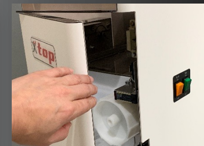
SAFETY It is safe because it stops when the front cover is opened.
