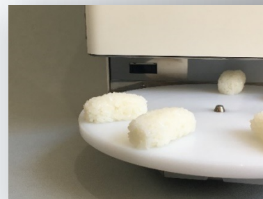
AUTOMATIC STOPPING automatic stop sensor indicates and stops the turning table if there are 6 Nigiri sushi on the table. 1 nigiri / 1.3 sec
